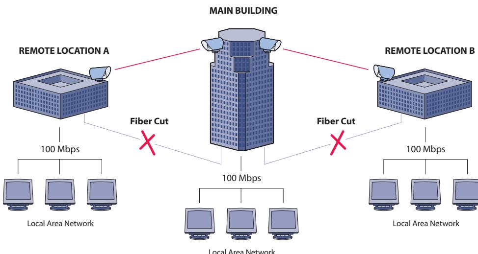
Optical Wireless solutions rapidly restore LAN connectivity with beams of light.
